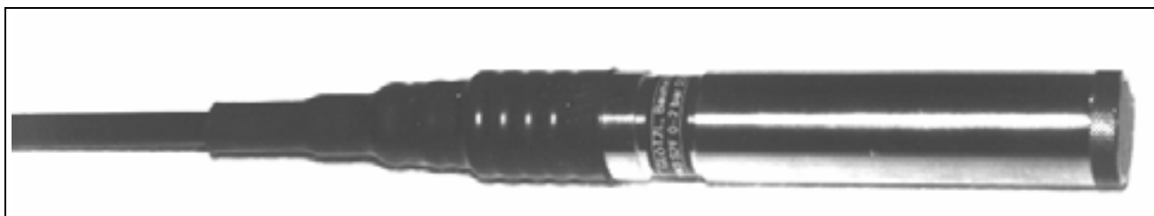
Figure: Pore water pressure transducer with front diaphragm
