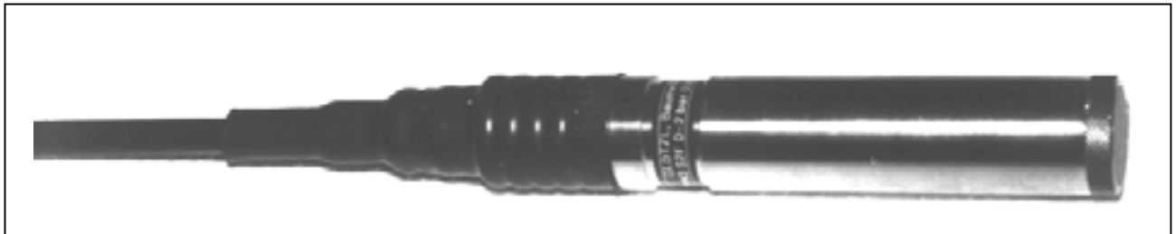
Figure: Porewater pressure cell with front filter stone
