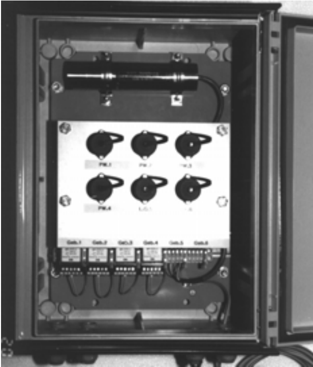
Hand operated distribution unit for 6 points with additional air pressure sensor Housing of polyester for wall or rod installation IP 66 Type AKVW 6/LS
