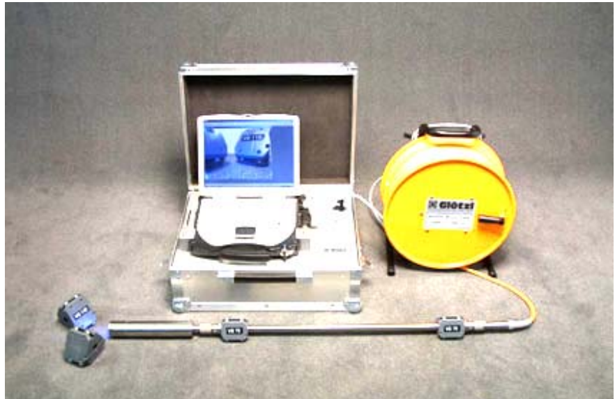
Figure 3 shows an autarkical video measuring system with video probe, guide adapter, cable reel and acquisition unit with notebook. The guide parts are exchangeable and thus can be adapted to the borehole diameter.
