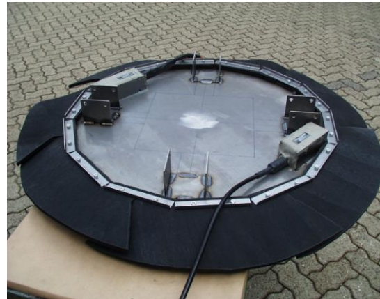
Fig.: Pile bottom cell, upper side, with cell, assembly bracket and microcell. rubber
