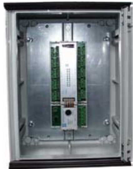
Multiplexer unit with 20 measuring points and control
